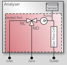
Inlet and zero are connected on a 3 ways electric valve. When the automatic zero is activated, the solenoid valve switches the flow cell on zero air. A pressure sensor takes the pressure of measured gas to compensate it and to give a flow indication.
